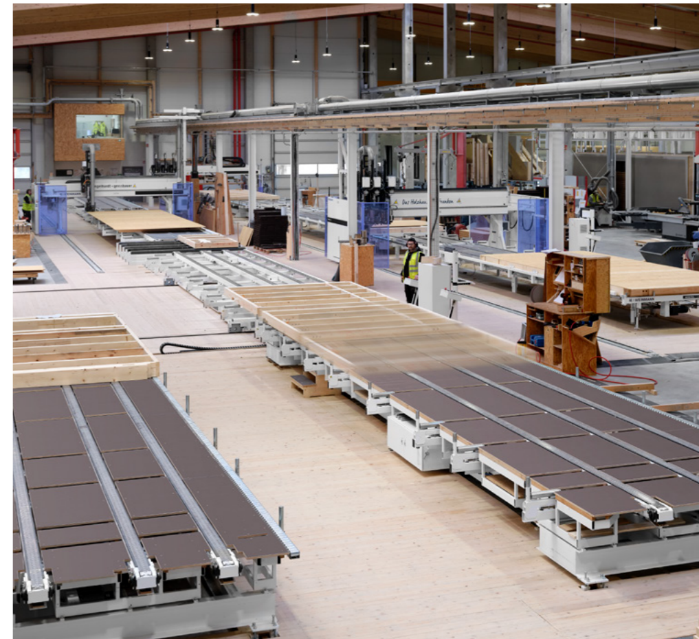
Pictures: On the production line, the frame work is created in parallel on two element tables and then processed by the multifunction bridge.
