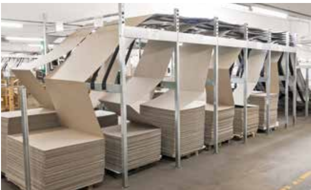
In the side-by-side operating mode, the carton feed compartment is extended by another web width, so that up to 12 web widths are possible in single access with a 6-compartment changeover system.
