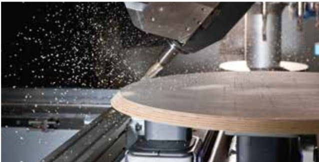
Chamfer trimming on a table top
