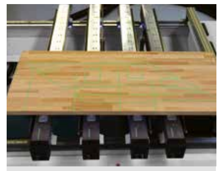
Laser projection of the clamping equipment and the workpiece contour for optimal utilization and simple positioning of unprocessed parts that cannot be aligned on the stops.
