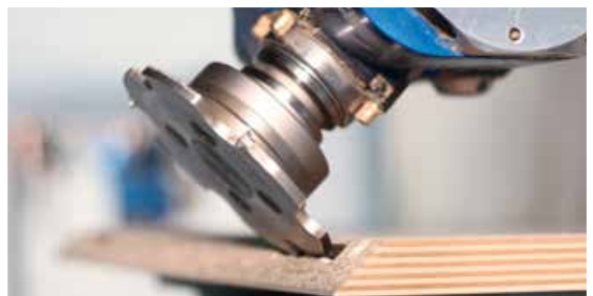
Cutting recesses for connecting fittings
