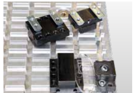
Aluminium matrix table with trapeze shaped grooves for interlocking and flexible fixing of all kinds of clamping aids
