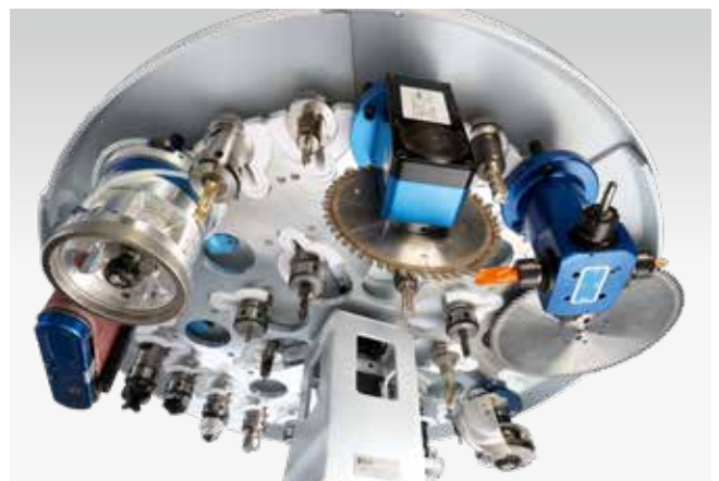
32-slot (24-slot) tool changer – arrangement of the tools in an inner and an outer ring. For tools and units with a diameter of up to 200 mm and saw blade up to 350 mm in diameter (in the outer ring).
