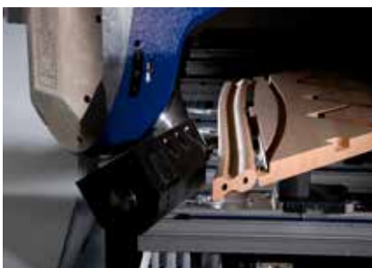
Paling holes at a tight angle
