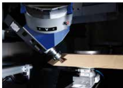
Trimming a burr connection for jamb/rail designs
