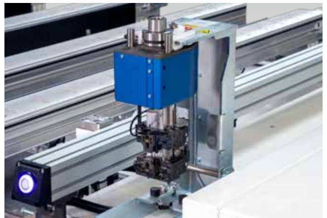
The tool transfer station allows the tool changer to be easily loaded and prevents errors.
