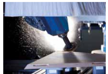
Trimming of angled grooves for panel connection
