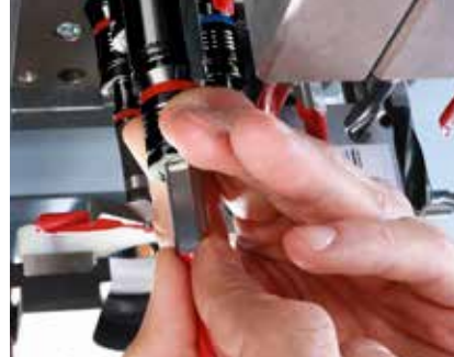
Patented quick-change system for a drill change without tools to reduce setup times.
