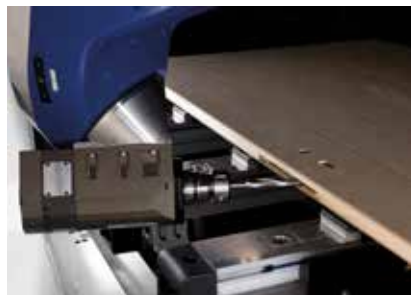
Trimming the lock casing
