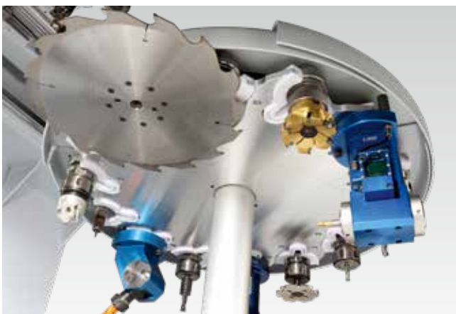
14-slot disc changer for tools and units with a diameter of up to 200 mm and saw blade up to 350 mm in diameter.
