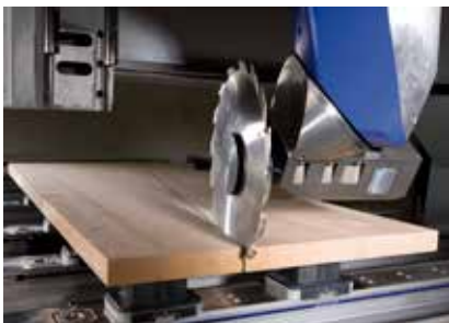
Separating cuts up to 110 mm in height
