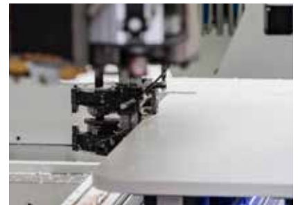
Perfect edge finish through traced combination flush trimming/scraper unit
