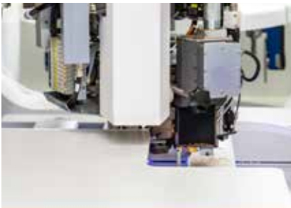
360° edge gluing with the powerEdge Pro Duo edge banding unit
