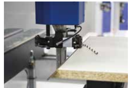
Scraper processing on the mitering edge
