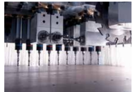
High-speed drilling technology with groove saw
