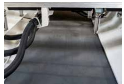
Chip transport For easy disposal of the offcuts and chips.
