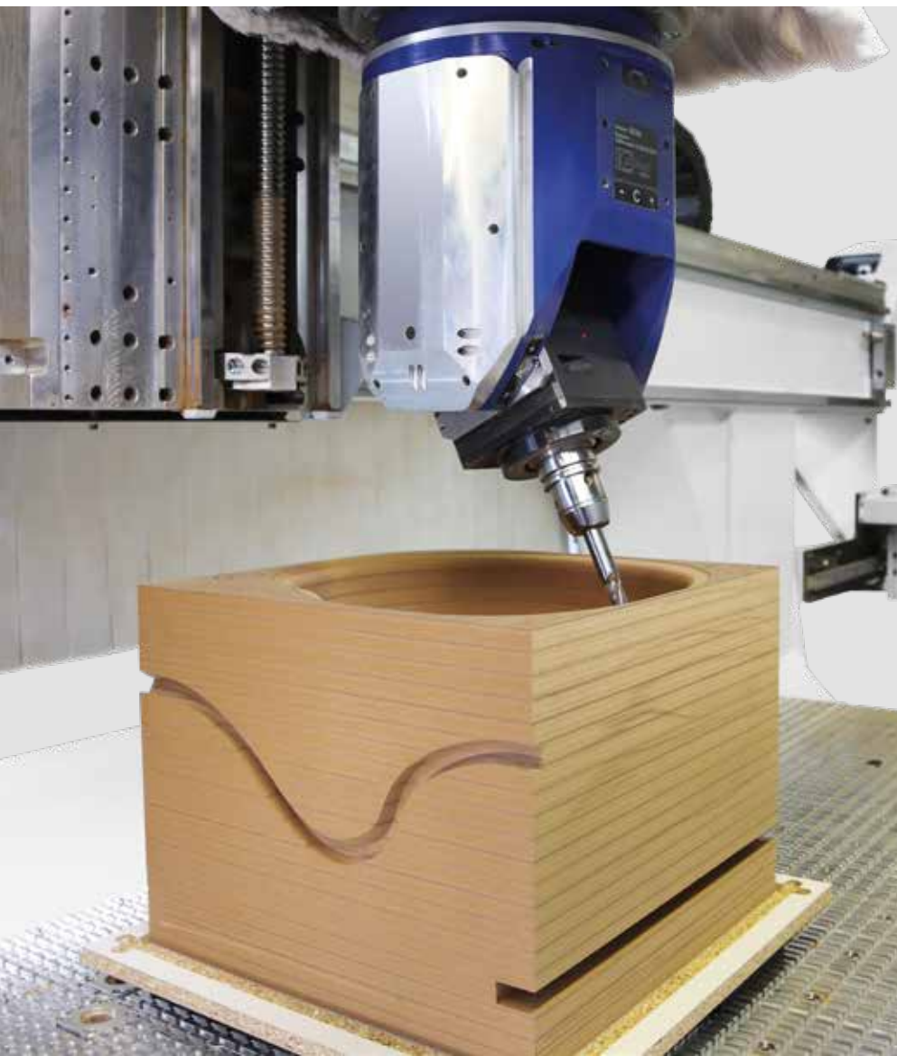
Trimming of components with a high Z height
