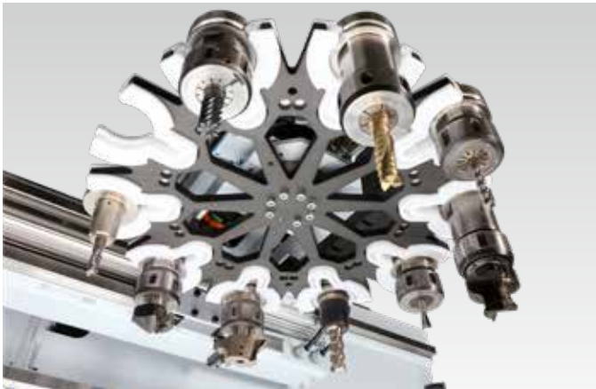
10-slot disk changer piggybacking on the spindle. Tool change during drilling or edge banding. For tools and units with a diameter of up to 180 mm.
