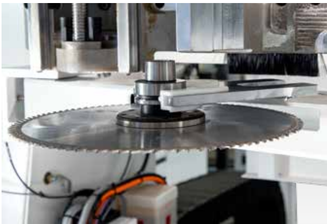
An additional pick-up slot for saw blades up to a diameter of 350 mm saves space in the tool changer. Can be freely combined with other tool change systems.
