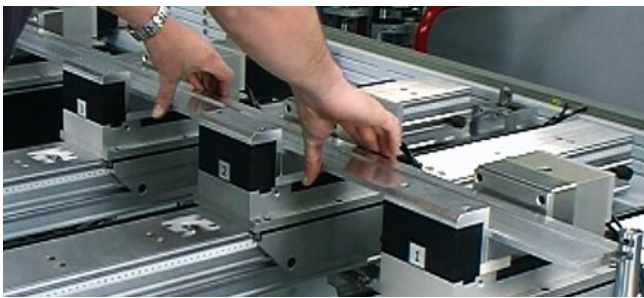
Special clamping elements for aluminum processing
