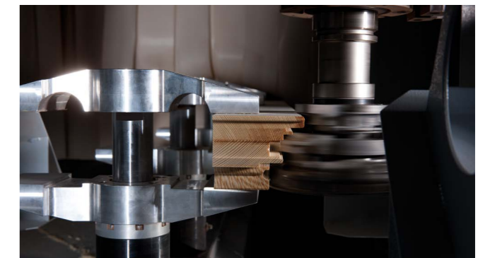
Liquid-cooled trimming spindles with vector control
