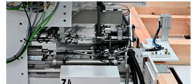
Screw unit for screwing frame works together.
