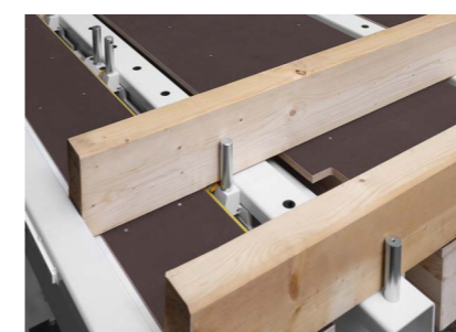
Roof/ceiling clamps facilitate insertion and fixing of roof rafters and ceiling beams.
