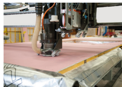
Processing gypsum plasterboard
